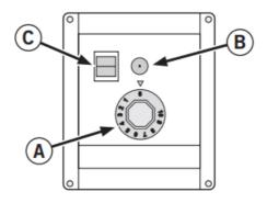
• A. Temperature Control Dial — used to set or adjust the well temperature. The higher the number the higher the temperature, the lower the number the lower the temperature. On models with no On/Off switch, the "0"
