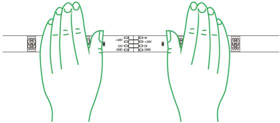
5. For corner setup, bend the strip and reinforce via clips; ( Notice: Avoid bending on LED beads.)
