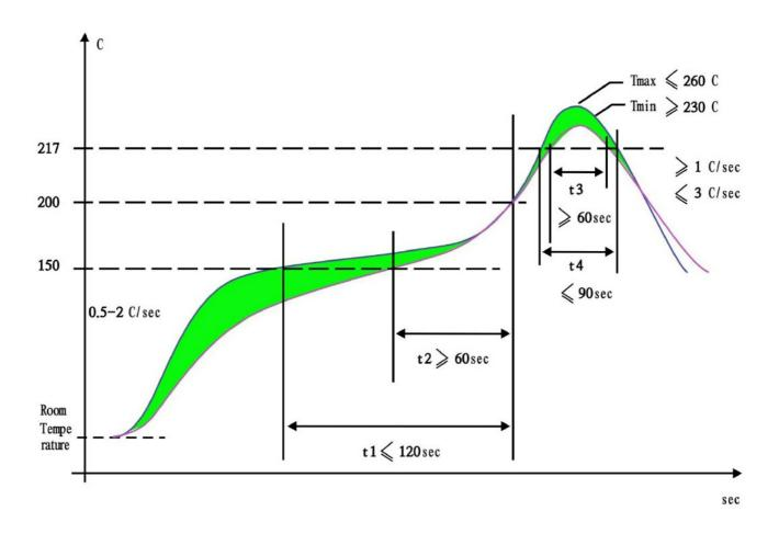
Lead-free reflow welding process parameters are shown in the following table.
