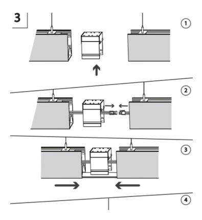
The connection bracket is not designed to handle the excessive load, caused by incorrect luminaire installation!
