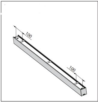
Modules should be parallel, aligned, without a gap in between before installing a connection bracket in order not to create excessive load! Use level to chek if modules are parallel
