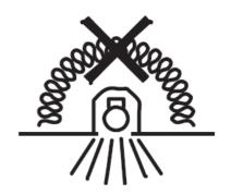
Install LED luminaire only in a clean room using gloves
