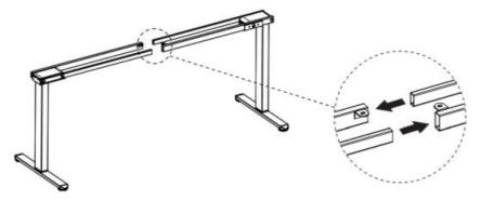
Secure Extension Connector (D) to the side of Crossbar With Plate (G) using M8x12mm Screws (S-C) and 5mm Allen Wrench (T-A).
