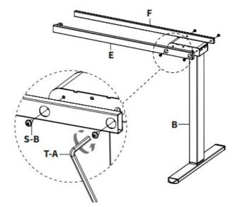
Slide crossbars of third leg assembly onto the existing assembly to form a corner frame shape.
