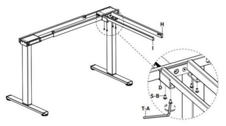
Assemble Inner Crossbar (F) and Outer Crossbar (E) to remaining Motorized Leg (B) using M6x14mm Screws (S-B) and 5mm Allen Wrench (T-A).
