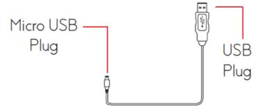
2. Insert the cable's standard USB plug into the USB port of a computer or suitable USB charging adapter. Then insert the cable's Micro USB end into the speaker's charging port. Charging in red light, Light off after full charge. into the speaker's charging port. Charging in red light, Light off after full charge.
