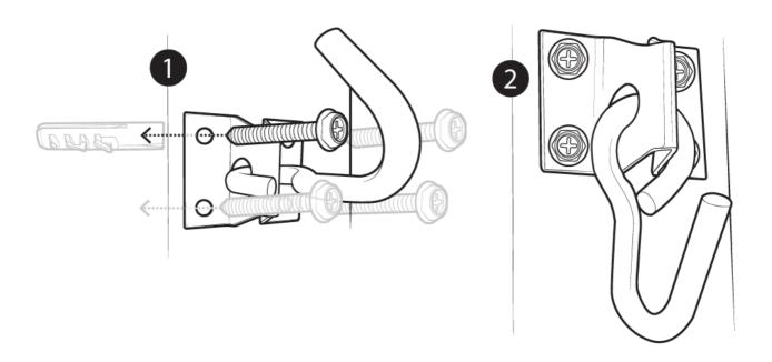
The best way to hang your hammock is with a Plate Hook. Screw the plate hook into a solid upright beam. Two fixed points are necessary for hanging hammocks. The ideal position for these points: 3-4 m apart, 1.8 m high. Ensure a nice loose curve 30cm off the ground when sitting in the hammock.
