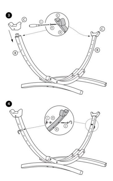
Do not tighten bolts until fully assembled.
