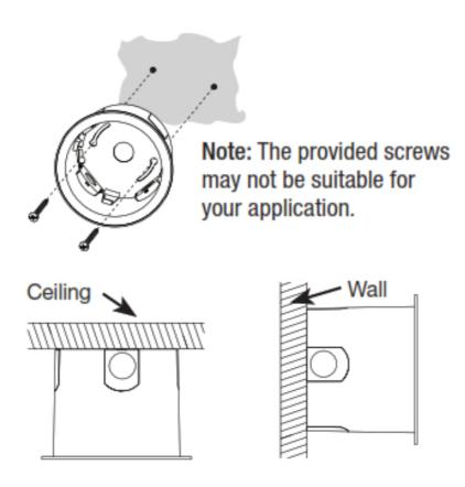
B. Alternate installation methods: Attach the surface-mount adapter to a Lutron-supplied US-style 101.6 mm x 101.6 mm junction box
