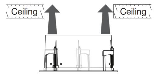
C. Using a Phillips head screwdriver, hand-tighten the brackets, clamping the adapter to the ceiling. DO NOT overtighten.
