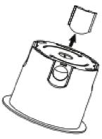
Attach the surface-mount adapter to the wall or ceiling using the included screws or appropriate screws that will securely mount the device.
