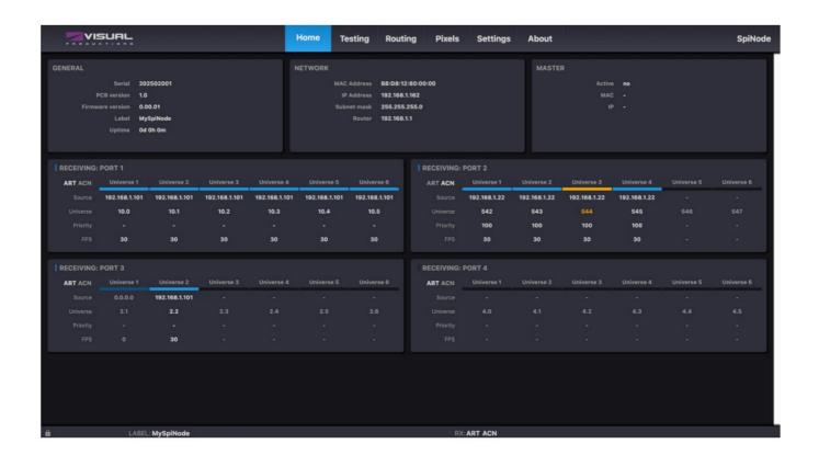
**GENERAL:** indicates general information about the SpiNode, like its serial number, the PCB version, the firmware version, the label associated with it and the uptime (time since the last reboot) of the unit.
