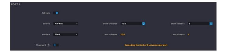
The SpiNode can receive up to 6 universes per port. However, if you patch the maximum number of pixels on one port and do not use 1 as a start address, you will need to receive 7 different universes.
