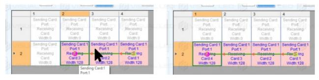
WHEN WE REACH THE END OF THE ROW WE CLICK ON THE TOP CABINET FOLLOWING THE PATH OF THE NETWORK CABLES ON THE SCREEN.
