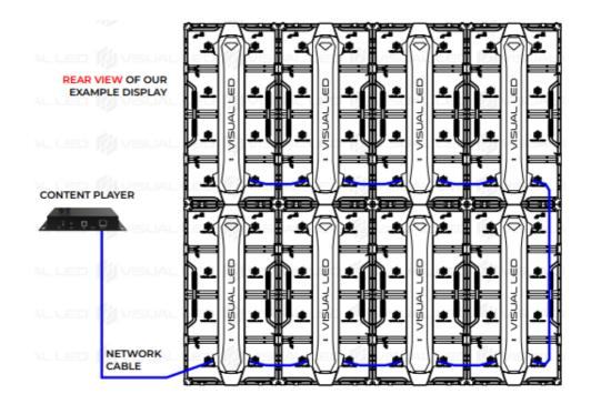
**IMPORTANT**: IN NOVALCT WE WILL SHOW THE DISPLAY DATA WIRING FROM A FRONT VIEW. THEREFORE, THE DATA WIRING ENTERS FROM THE LOWER RIGHT FRAME.
