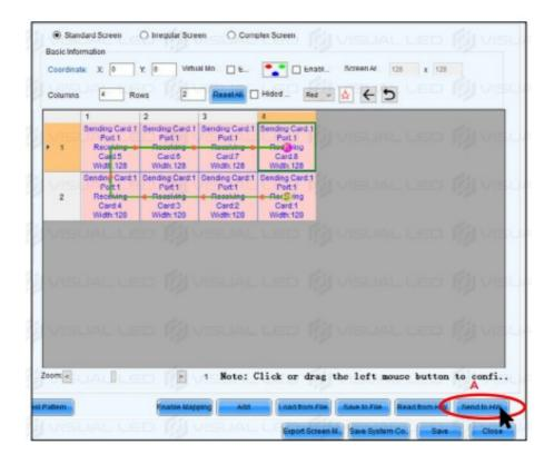
AFTER DRAWING THE DATA WIRING ON THE CABINETS, WE WILL SEND THIS CONFIGURATION TO THE SCREEN.
