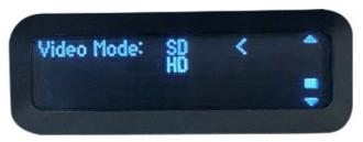
When SD video is selected it is possible to PTZ the SD video frame around within the higher resolution HD frame.
