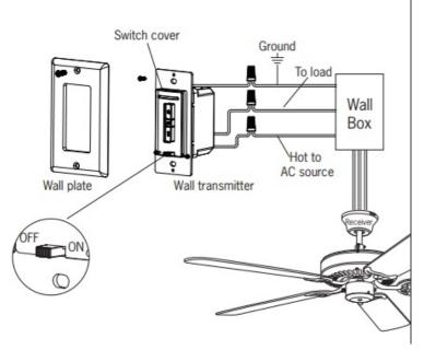
Install the wall transmitter to outlet box using machine screws provided.
