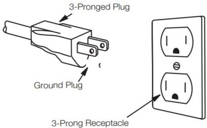
The electrical requirements are a 120 volt 60 Hz, AC only, 20 amp. It is recommended that a separate circuit serving only the oven be provided. The oven is equipped with a
