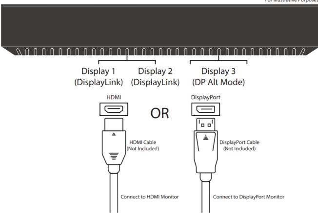
Display 1 and 2 function via DisplayLink when connected with USB-A or USB-C. Display 3 is supported via USB-C DP Alt Mode and will only output video when connected via USB-C.
