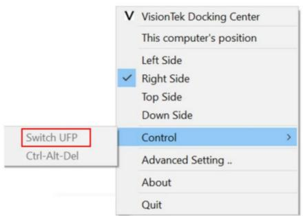
When the Hub connects to two PCs, devices under the hub will be recognized and enumerated by the Master host, for example, the storage devices will only be shown on the Master PC, while the other PC is set as the slave PC. Switch UFP function will allow users to switch the role of Master and Slave PCs.
