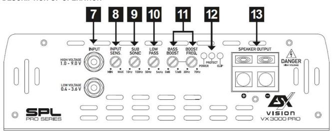
7. There are two RCA inputs on the LINE INPUT, each of which is controlled in mono. The input LOW VOLTAGE is suitable for low level signals from 0.4 to 3.6 volts. At the input HIGH VOLTAGE you can connect a high level signal from 1.0 to 9.0 volts, such as that provided by a DSP.
