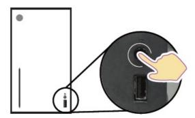
3. 3. Press the ")))" buttons on both the controller and console, the indicator will fast flash to enter the pairing mode. After connection, the indicator will always be on.
