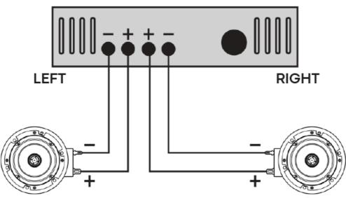
Push the terminal posts and insert the cable.
