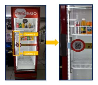
Smart Vision is installed completely aligned with the inner edge of the door without obstructing the door's close. Smart Vision must be installed inwards from the cooler door frame and should not touch the
