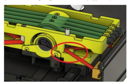
4. Slide the center of the elastic rope into the slot to ensure that the YOKO<sup>neo</sup> is completely centered in its pitch range of motion. For the pitch axis to be centered properly, the two marks indicated in amber color must align, as shown below.
