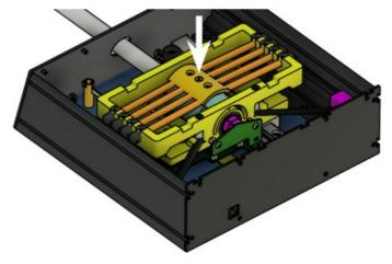
4. Center the dumbbell by rotating the yoke in both directions until the dummbell is level when at its neutral position.
