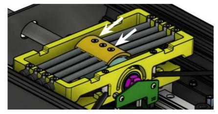
6. Replace the central M4x15 screw (J) with the original (shorter) screw in the center.
