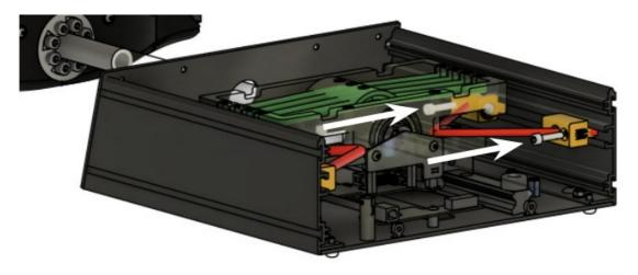
3. Slide out the elastic rope from its slot until as shown below to remove it from the  $YOKO^{neo}$ .
