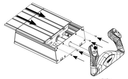
2. Place the back plate and screw in the 10 screws located at the back of the YOKOneo using the n4 Allen Key.
