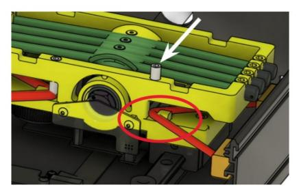
2. Unscrew the 2 indicated screws with the n5 allen key.
