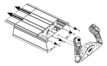
Once the interior of the YOKO<sup>neo</sup> is exposed, you can modify the Elevator or Ailerons control stiffness by following the next steps.
