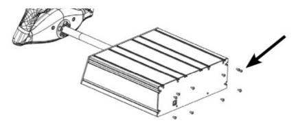
2. Unscrew the 4 screws from the front plate of the  ${}^{YOKO^{neo}}$  indicated below and slide the upper plate out, exposing the interior of the  ${}^{YOKO^{neo}}$ .
