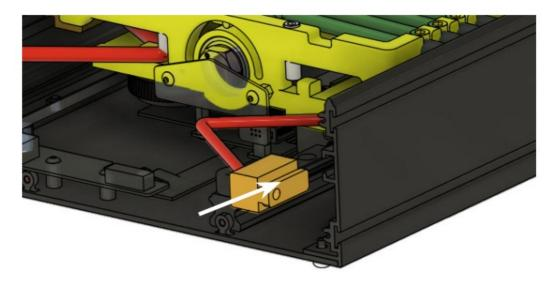
2. Secure the 2 elastic rope supports by screwing in the two indicated screws below
