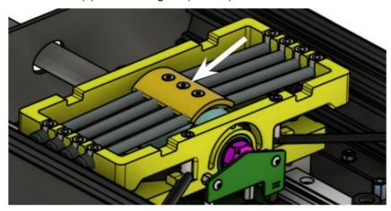
After adding/removing the elastic ropes to your liking, you must cover the yoke by reversing the process you did to access the interior:
