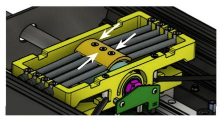
2. Add/remove the necessary elastic ropes according to the desired resistance following the Table 2.2. To do this, you will need to screw/unscrew the indicated screws of the elastic rope you wish to add/remove.
