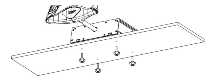
To screw in the clamping knobs (D), you will need a cutout that matches the measurements depicted in the blueprint below.
