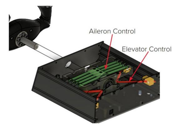
By default, the YOKO<sup>neo</sup> comes with 2 aileron control elastic ropes and one 6 mm elevator control elastic ropes installed. The user can choose between the three stiffness options depicted in Table 2.2.
