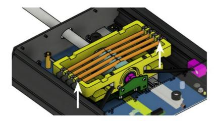
3. Place the cover back into position and screw in only the central indicated screw, making sure it is not tight. For ease, it's better to use the longer J screw (M4x15).
