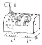
3. Insert the Assembly's guides on the TRIMS neo's slots as indicated below.
