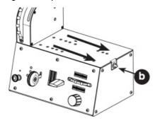
2. Unscrew the TQ's rubber feet (if applicable), align the holes from the Adapter and TQ and attach the TQ into the Adapter with the screws provided with it as shown below.
