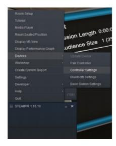
The second way to access the bindings is on the desktop. This opens the same interface. To access it here, click the hamburger menu on the SteamVR app; Select Devices and then Controller Settings.
