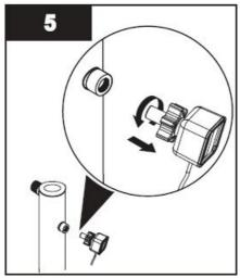
• Install the new sensor to the UV chamber.
