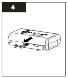
• Remove the old sensor from UV chamber.
