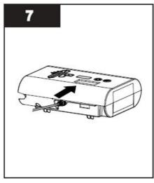
• Restore power and connect the other devices such as a solenoid, junction box, and remote alarms.
