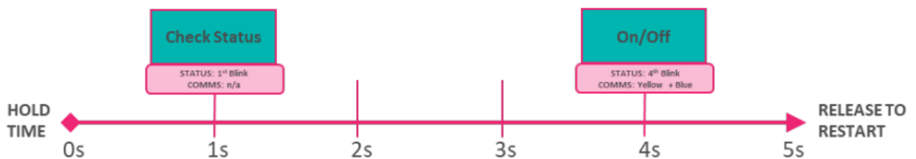
Figure 3 Flow Diagram for Cycling System Status with Magnet
