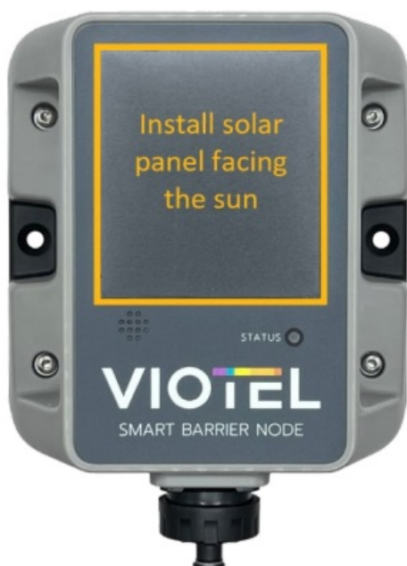
Figure 3 Required orientation of the solar-powered node
