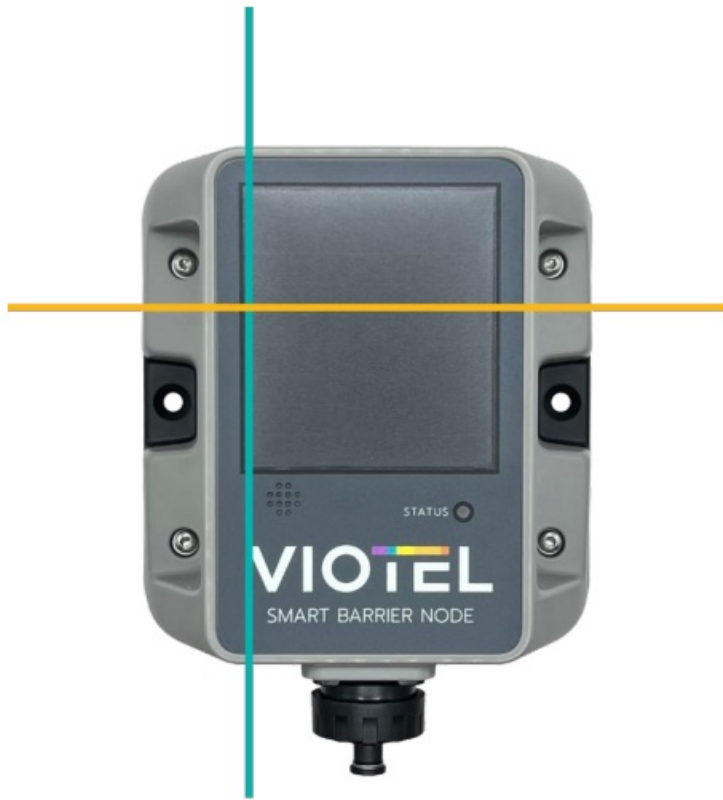
Figure 5: Photo highlighting location of the magnet for Smart Barrier Node
