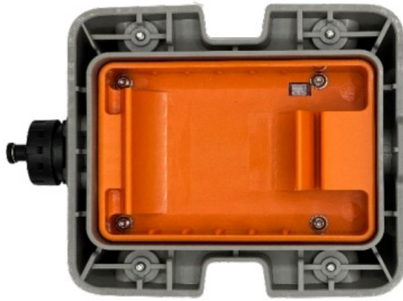
Figure 8 Tiltmeter with battery removed
