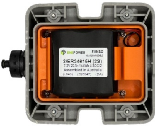
Figure 7 Tiltmeter with backing plate removed
