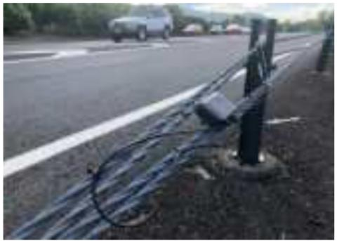
The Viotel Smart Barrier node features a unique patented design for quick installation on wire rope barriers and fences. The node measures the tension of the wires, and monitors the barrier for impacts. The Smart Barrier node uses an integrated solar panel and rechargeable battery, and an internal Cat-M1 modem for communications. The barrier status is uploaded regularly, and whenever an impact is detected.
