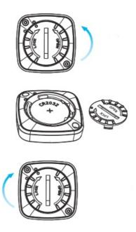
1. Open the battery cover by turning it in the direction of the arrow.
