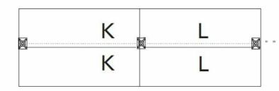
Make sure that the perforation of the rear panel does not remain between the union of the pieces K-L, so that they do not separate.
