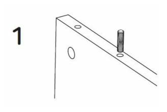
Put in the dowel inside the indicated hole and softly hit it until it's fully inside
