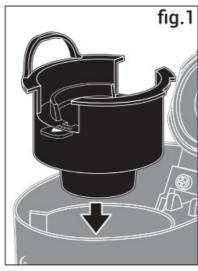
3. Insert the capsule basket into place by aligning the front of the capsule basket pointing to the front of the unit (see fig. 1). The capsule basket handlew ill be positioned to the left of the pod coffee maker.
