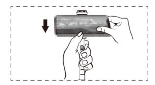
**Step 2:** Hold the handle sleeve and use the other hand to push the aluminum alloy telescopic arm back from the top cap.
