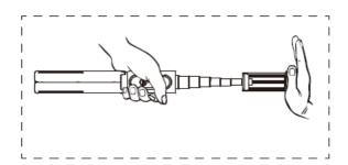
**NOTE:** if you open the tripod, the tripod will close automatically when push back the aluminum alloy telescopic arm. Manual opera on is prohibited.
