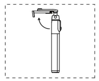
**Step 2:** Rotate the phone holder around the tripod to align with the front of the tripod
