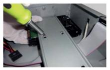
2. Connect the power and data cables and install the other three HDDs according to above-mentioned method and install back the upper mounting bar.
