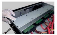
3. Install the upper four HDDs and install back the cover.
