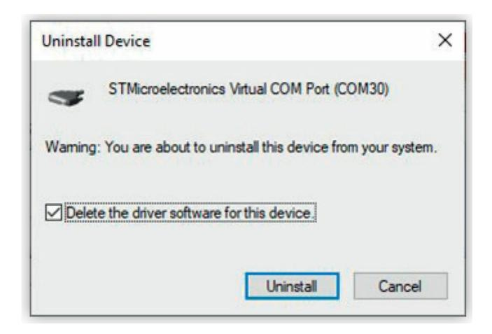
If the previous tests had a negative outcome and there are no hardware problems, it is likely that the driver is the cause of the malfunction; in this case, reinstall it.
