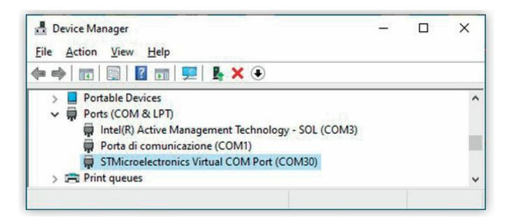
If the reader remains in the "Not connected" state, check that the reader is connected to the PC and recognised by it.
