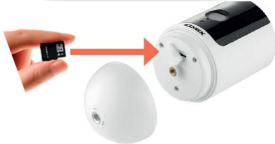
Unscrew the dome cover to access the SD card.
