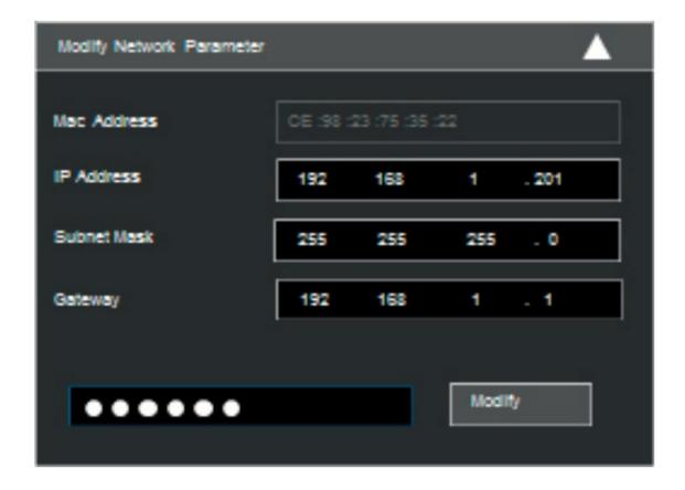
For example, the IP address of your computer is 192.168.1.4. So the IP address of the camera shall be changed to 192.168.1.X.
