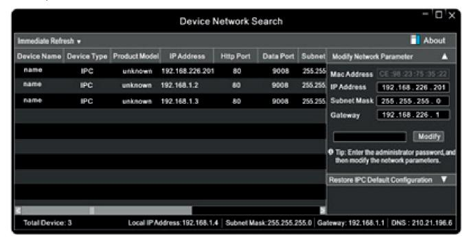
3. Modify the IP address. The default IP address of this camera is 192.168.226.201. Click the information of the camera listed in the above table to show the network information on the right hand. Modify the IP address and gateway of the camera and make sure its network address is in the same local network segment as the computer's. Please modify the IP address of your device according to the practical situation.
