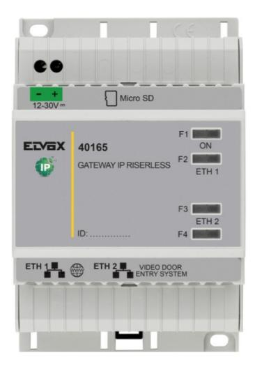
IoT Gateway for connection to the Vimar Cloud of an IP video door entry system. Once the necessary licences have been installed, it provides the video door entry service up to a maximum of 100 virtual apartments. Up to 5 instances of APP can be associated with each apartment. Installation on DIN rail (60715 TH35), occupies 4 modules size 17.5 mm.
