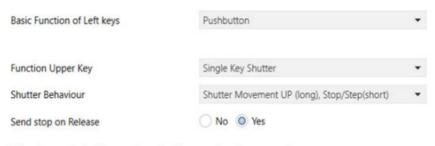
"Single push button roller shutter control" parameters
