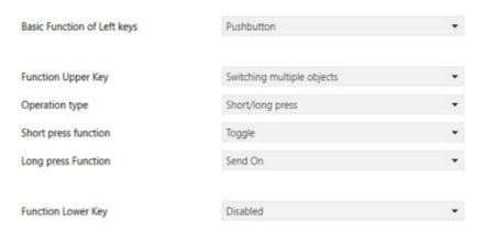
"Switching several objects/Short-long press" parameters with Toggle and ON/OFF" options
