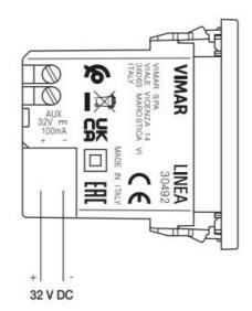
Graphic representation of the Linea series. Position of terminals, wiring, and functions is also identical for Eikon, Arké, and Plana.
