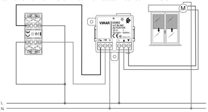
**N.B.** Graphic representation of the Linea series. Position of terminals, wiring and functions also identical for Eikon, Arké, Idea and Plana.
