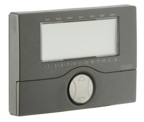
Electronic timer-thermostat for ON/OFF ambient temperature control (heating and air conditioning), daily/weekly programming, class I temperature control device (contribution 1%), change-over relay output 5(2) A 250 V~, powered by batteries AA LR6 1.5 V (not supplied), wall mounting.
