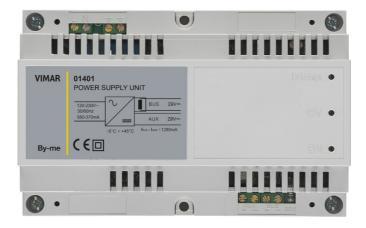
Power unit with output 29 V d.c. 1280 mA, power supply 120-230 V~ 50-60 Hz, with decoupling coil, installation on DIN rails (60715 TH35), occupies 8 modules.
