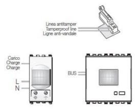
4. Fix the detector to the cover designed to accomodate the equipment.
