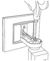
7. Insert and fix the microswitch cardinside the upper cover of the orientable support (only for 20485-19485-14485).
