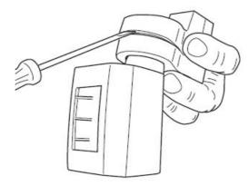
2. Unscrew the screw blocking the joint until the cover designed to accommodate the equipment is released.
