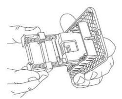
2. Fix the supporting frame to the flush mounting box, apply the cover plate and fix the orientable support using the delivered screws.
