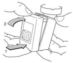
6. Orient the detector as desired and fasten the screw blocking the joint.
