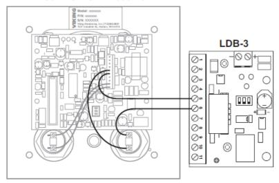
The "Disable" input can be connected to a remote switch, contact closure, etc. for deactivating the LDB-3's internal relay. This can be useful to turn off the controlled device (strobe light, camera, etc.) Use the diagram shown at the right. If the relay has been activated by ringing, the switch will deactivate the relay and ringing must stop for a minimum of 6 seconds before the relay can be re-activated from a new incoming call.
