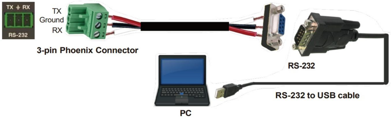
Then, open a Serial Command tool on PC to send ASCII commands to control the product. The ASCII commands list about the product is shown as below
