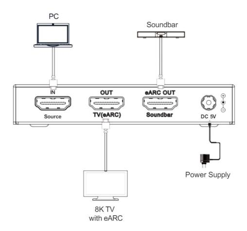
**Note:** When eARC function is turned on, the audio signal of Soundbar is the audio returned from 8K TV. When eARC function is turned off, the audio signal of Amplifier is from the HDMI input source.
