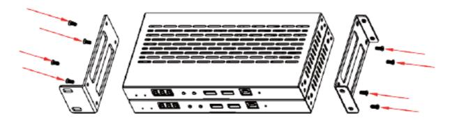
**Step 2:** Fix two 1U rack panels on another two stacked products in the same way, then use screws to fix two 1U rack panels together, as shown in the figure below:
