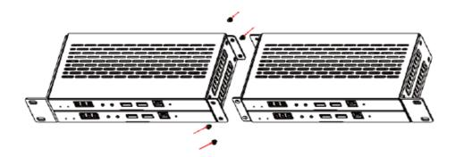
**Step 3:** Fasten screws between two 1U rack panels, so that four products are mounted in a 1U rack, as shown in the figure below:
