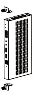
**Step 2:** Insert the product with mounting ears into a 6U rack (up to 10 units can be installed vertically), as shown in the figure below:
