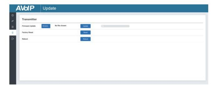
Click "Browse.." to import the upgrade file and click "Update" to start the upgrade. There will be a progress bar prompt during the upgrade process. When the progress bar reaches 100%, it indicates the upgrade is successful, and the device will be restarted automatically. Clicking "Reset" can reset the device to factory default settings. Clicking "Reboot" can reboot the device.
