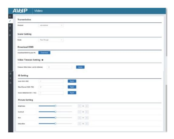
Transmission Protocol: You can select "UDP unicast" or "UDP multicast" (UDP multicast by default).
