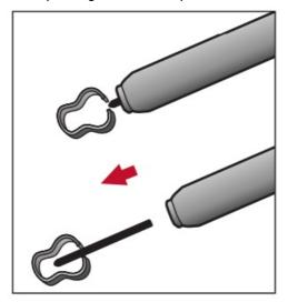
2. Insert a new pen tip into the pen and push the tip in until it stops and is held firm.
